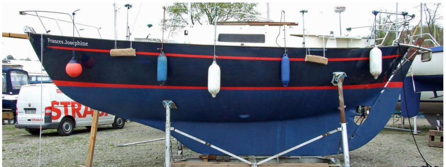
FRANCES JOSEPHINE in a cradle after the keel modification. The flatter sole of the keel is clearly visible.
