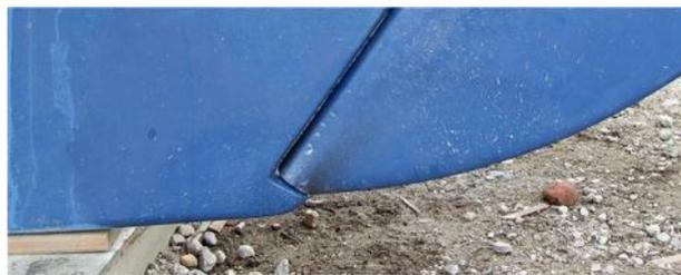
The photograph on the left shows a small heel. It is made from a piece of hardwood, encapsulated by epoxy and fibreglass mat.
