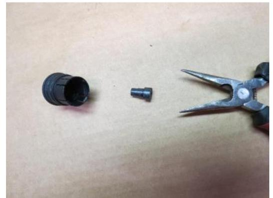
Once the magnet assembly is removed, push the inside end of the shaft. Both bearings and the shaft will push out easily. If they are not coming out, recheck that the securing dimples are fully removed.
