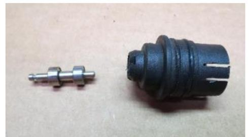
The shaft will probably have some dirt/debris/rust on the surface, so I chucked up the shaft using the middle area where the bearings don't ride using my battery drill. Holding the emery cloth or super fine sandpaper I cleaned both ends of the shaft.
